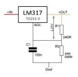
The LM317 (pos.) and LM337 (neg.) voltage regulator IC's are champions in regulating behaviour for many years, capable of delivering up to 1500mA in TO220 variants. In the replacement modules we present here, we use small and hard to find SMD TO253-3 types.
